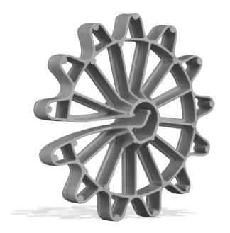
Spacer wheels are a simple and secure way to support reo bars and mesh to provide the required concrete cover. ConForce polyethylene spacers are easy to fit. They securely clip onto the steel bars and stay in place when vibrated.
