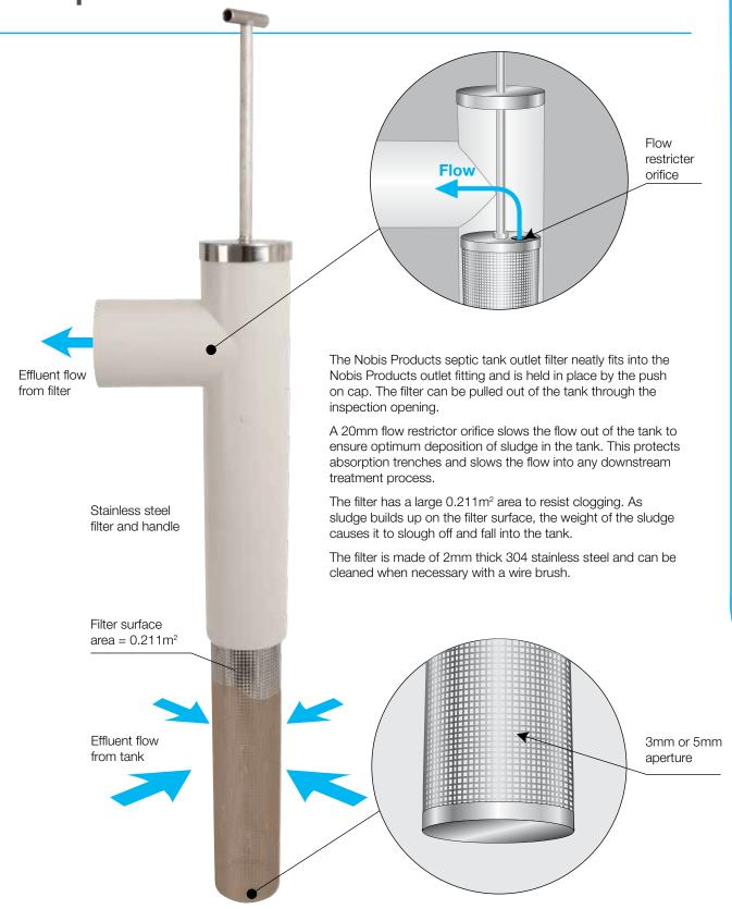
**Stainless Steel Septic Tank Outlet Filter**
